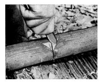
The finished triangular cut should be even, and as smooth as possible, but not extend beyond the midpoint of the timber. The notch is ready for fitting a tapered triangular end of the second timber.
