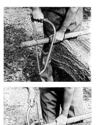
Then make a cut an angle of approximately 90 degrees, starting from the same initial cut opening. Make the cut to the same depth as the diagonal cuts. Multiple cuts can be made to make it easier to clean out the open area of the joint.
