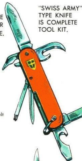
JACKKNIFE HAS BLADES AT ONE END ONLY, PEN-KNIFE AT BOTH ENDS.
