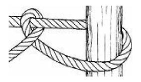
Wrap the line around the post or staff, and pass the working end of the cord thru the opening.
