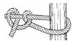
Wrap the line around the main strand of the cord and form a second loop, passing the end of the cordage thru the eye ensuring that the end exits in opposition to the entry of the first loop. Tighten and dress the knot.
